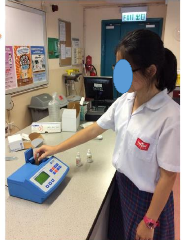
After 3:30 mins, read the concentration of ammonia
